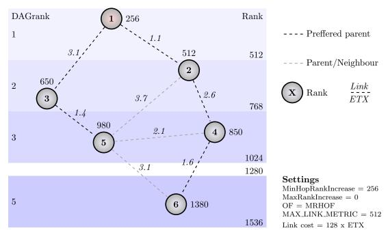
Figure 3.7: DODAG with ranks determined from ETX using the OF MRHOF.
