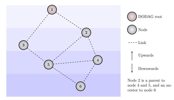
Figure 3.4: Example DODAG (a DAG would, strictly speaking, require directed edges, but these are left out from the figure as it does not include a specified sender/receiver path).
