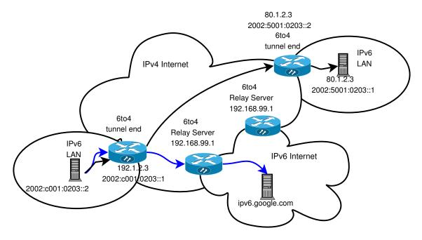
Figure 2.3: 6to4 Tunneling. Blue lines show 6to4 host to native IPv6 communication, black lines show a 6to4 to 6to4 path.
