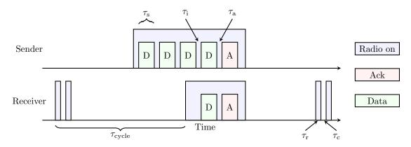
Figure 3.3: ContikiMAC RDC mechanism.
