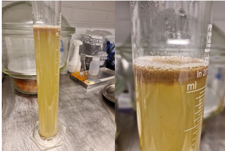
Figure 26: Extracting oil from pickling
