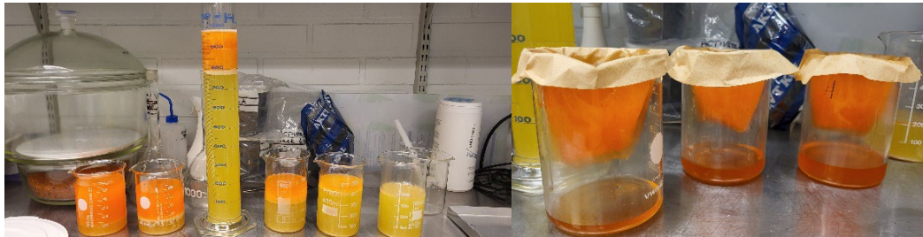
Figure 43: Cleaning process of the extracted oil, salmon
