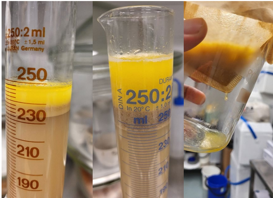
Figure 4242: Cleaning process of the extracted oil, pike
