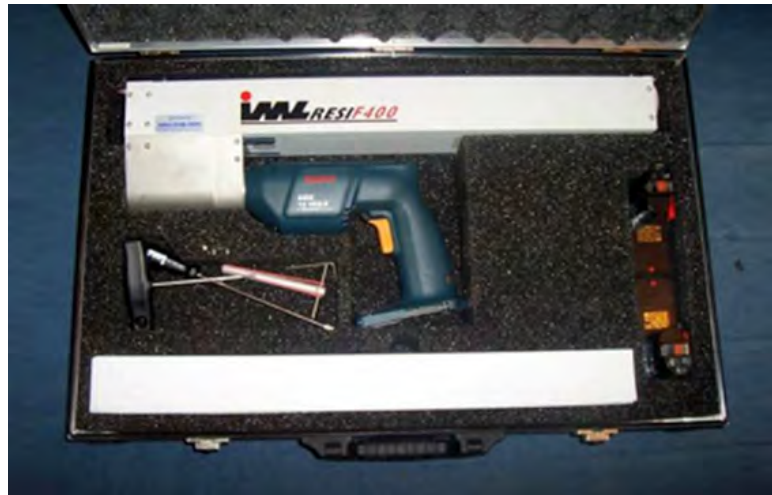
Figure 3.13. Micro drilling apparatus.
