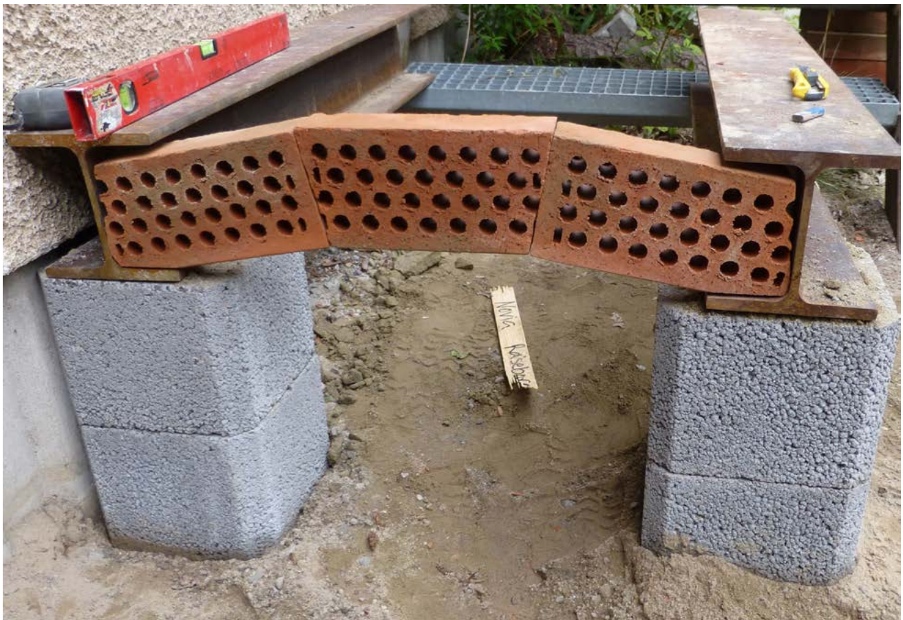
FIGURE 2.21. The shape of each brick was carefully measured and cut to make a flat vault. Photograph by Kirsti Horn.
