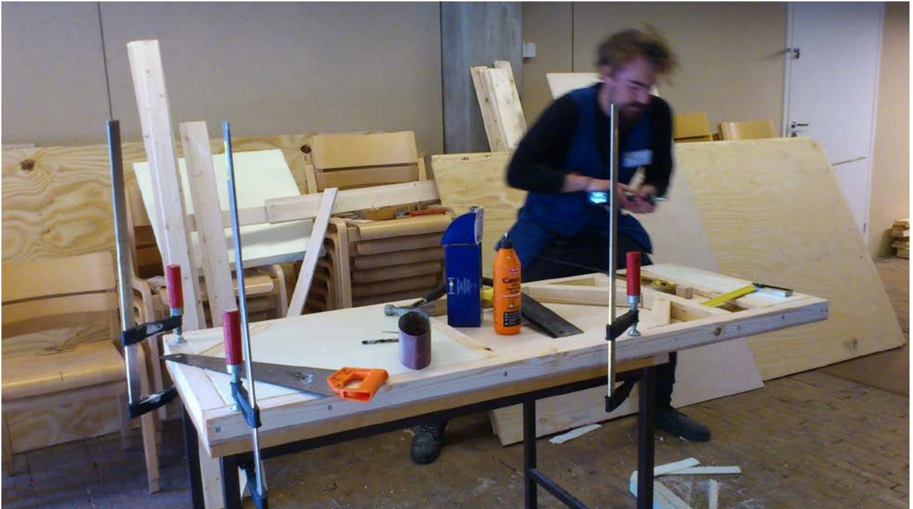
FIGURE 4.4. The plywood is being glued onto the framework of the door. Photograph by Sanna Svensson.
