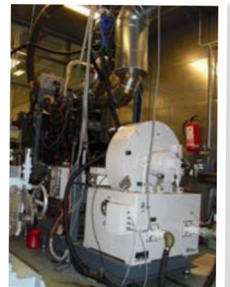
The fuels were tested in a AGCO Sisu Power 44CWA Non-road diesel engine in the engine laboratory in Techno-bothnia.
